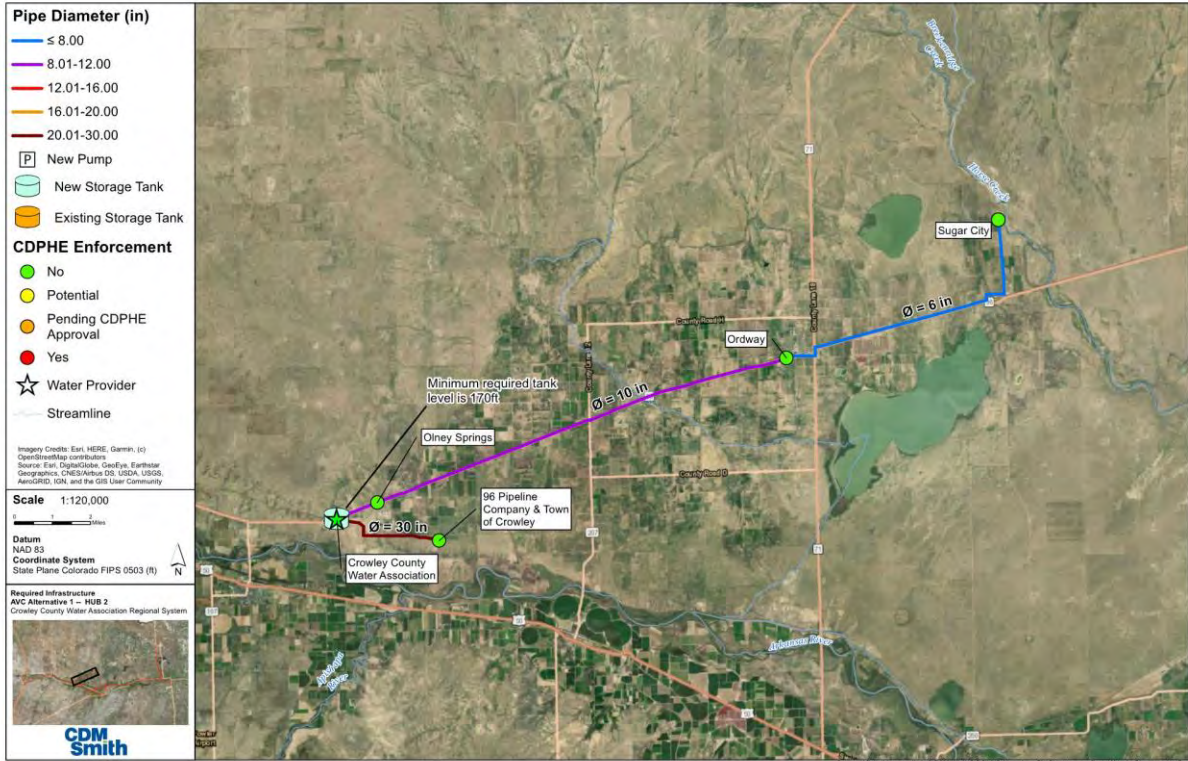
Figure 4-13. Alternative 1 Crowley County Water Association Regional System Participant Delivery Locations and Conduit Routes
