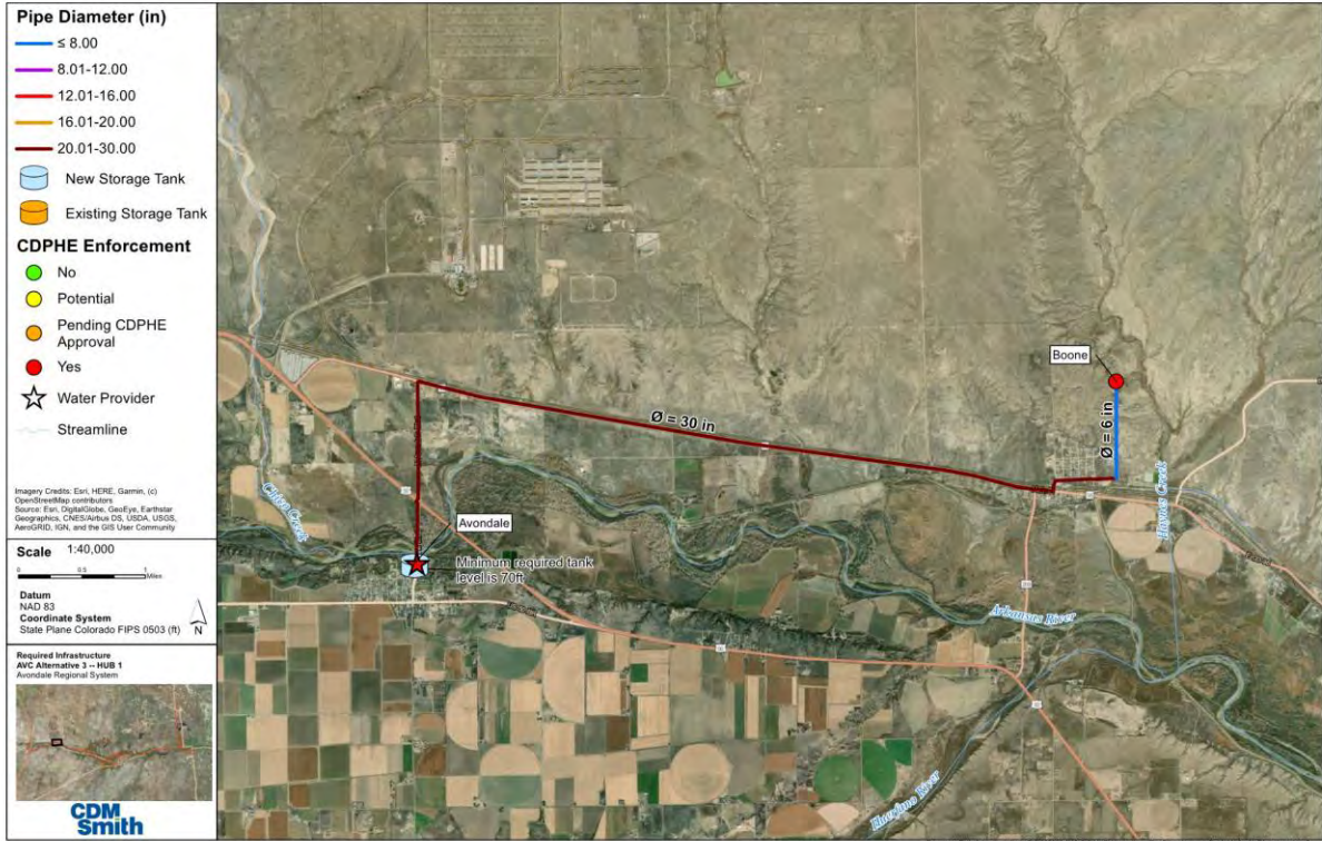
Figure 4-33. Alternative 3 Avondale Regional System Proposed Participant Delivery Locations and Conduit Routes
